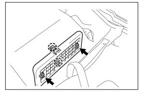
5. Remove the bolt and rear seat belt assembly inner NO. 1.
