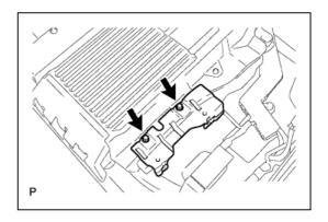
7. Remove the 2 bolts on each battery carrier duct and remove the battery carrier ducts LH, RH, and CENTER.
