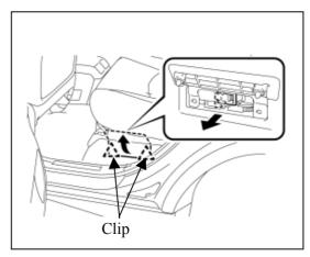
2. Carry the removed service plug in your pocket to prevent other staff from reinstalling it while you are dismantling the vehicle.
