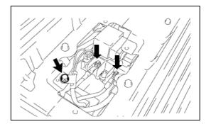
10. Disconnect the wires from the battery cooling blower, battery voltage sensor, and HV
