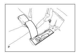
6. Remove the 2 bolts and battery carrier bracket.
