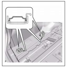
(2) Remove the 2 bolts and 2 rope hook assemblies.
