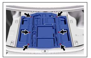
(3) Disengage the 3 guides and remove the luggage compartment trim box.
