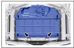
(6) Hold the areas shown in the illustration and remove the HV battery.
