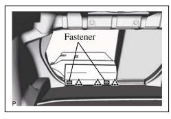
(3) Disengage the 5 fasteners.
