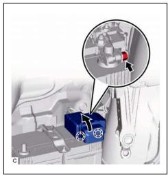
(3) Remove the nut and battery clamp sub-assembly.
