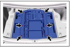
(2) Disengage the 3 guides and remove the luggage compartment trim box.
