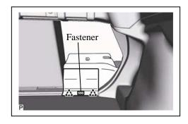
(3) Disengage the 5 fasteners.
