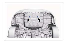
(2) Remove the 2 battery drain plugs as indicated by the arrows, in the order shown in the illustration.
