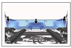
(2) Disengage the 6 clips to remove the rear luggage compartment trim cover.
