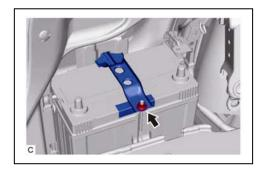
(4) Remove the bolt and battery hold down clamp sub-assembly.
