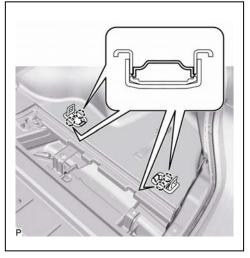
(2) Remove the 2 bolts and 2 rope hook assemblies.
