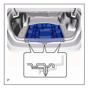
(4) Remove the 3 nuts and No. 5 HV battery shield panel from the HV battery.
