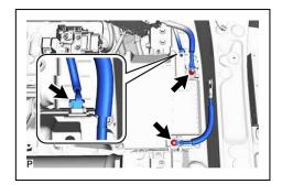
(3) Loosen the 2 nuts and disconnect the connector from the sub-battery module assembly.
