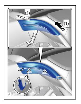
d) Place your hand at the position shown in the illustration and pull in the direction indicated by the arrow to detach the clamp and claw.
