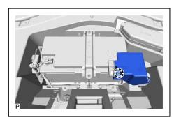
(2) Disconnect the clamp spring assembly of the positive(+) auxiliary battery terminal from the auxiliary battery.
