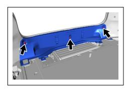
(2) Detach the clip and guide and remove the rear floor finish plate.
