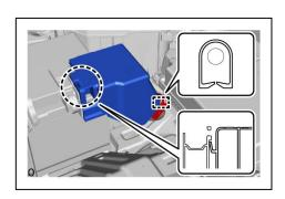
(2) Remove the nut and disconnect the HV floor under wire.
