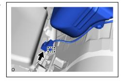
(2) Remove the 5 nuts, detach the clip and remove the rear cooling unit.
