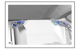
(4) Pull the rear outer belt assembly LH and rear center seat outer belt assembly out of the room partition board assembly LH and remove the room partition board assembly LH.
