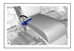
(2) Place your hand in the position shown in the illustration and lift the rear center seat cushion assembly in the removal direction and detach the hook.
