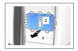
(2) Lift the door armrest cap in the direction indicated by the arrow shown in the illustration to disconnect it, and then secure it with adhesive tape.
