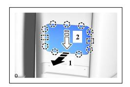
b) Lift the door armrest cap in the direction indicated by the arrow shown in the illustration to disconnect it, and then secure it with adhesive tape.
