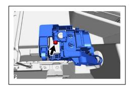
(4) Remove the 2 nuts and battery clamp sub-assembly.
