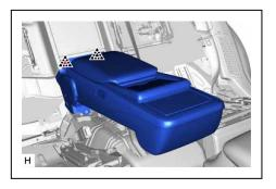
(6) Remove the 2 nuts and rear center seat armrest assembly.
