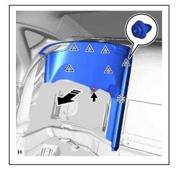
(3) Detach the claws and guide and remove the belt guide of the rear outer belt assembly RH.
