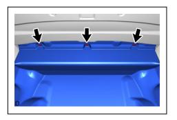
(2) Using a clip remover, remove the 3 clips
