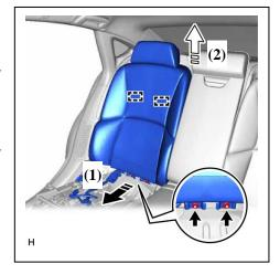
(13) Using a clip remover, detach the clip and remove the rear seatback assembly RH.
