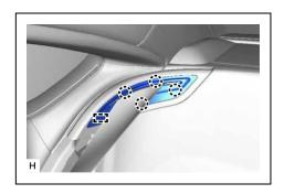
(4) Pull the rear outer belt assembly RH out of the room partition board assembly RH and remove the room partition board assembly RH.
