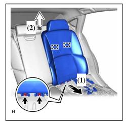
(13) Using a clip remover, detach the clip and remove the rear seatback assembly LH.
