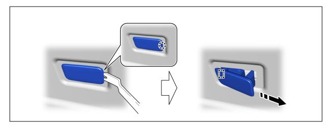
(3) Disconnect the connector and remove the luggage compartment light assembly.
