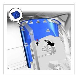
(3) Detach the claws and guide and remove the belt guide of the rear outer belt assembly LH and rear center seat outer belt assembly.
