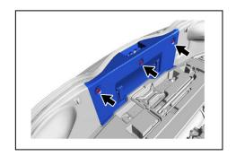
(2) Detach the clips and guides and remove the rear floor finish plate.
