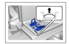
(2) Remove the bolt and rope hook.
