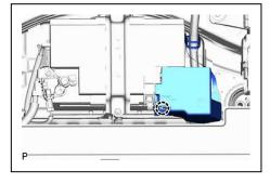
(2) Loosen the nut and disconnect the cable from the positive (+) auxiliary battery terminal.
