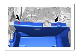
(2) Remove the 2 clips and No. 1 hybrid battery intake duct.
