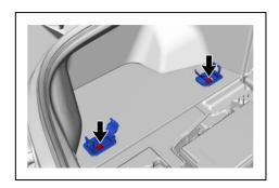
(3) Pull the entire luggage compartment trim cover LH to the rear while bending inward (in the direction of the arrow) to remove it.
