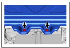
(2) Push the lever and remove the rope hook.
