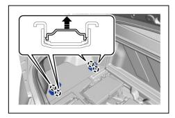
(2) Remove the 2 bolts and 2 rope hooks.
