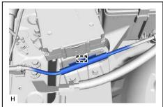
(4) Remove the 2 bolts, nut and fuel pump control ECU bracket from the vehicle body.
