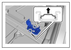
(2) Remove the bolt and rope hook.
