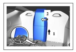
c) Remove the strap fixing bolt and rear seat side garnish.
