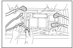
5. If the service plug grip cannot be removed due to damage to the vehicle, remove the **J/B D-B** Fusible Link (40 A).
