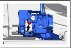
(3) Remove the 2 nuts and battery clamp sub-assembly.
